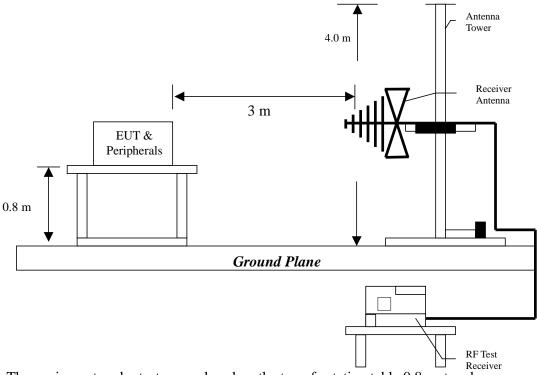
The equipment under test were placed on the top of rotation table 0.8 meter above ground plane.
