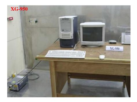
**Appendix B2: Conducted Emission Test Set-up (rear)**
