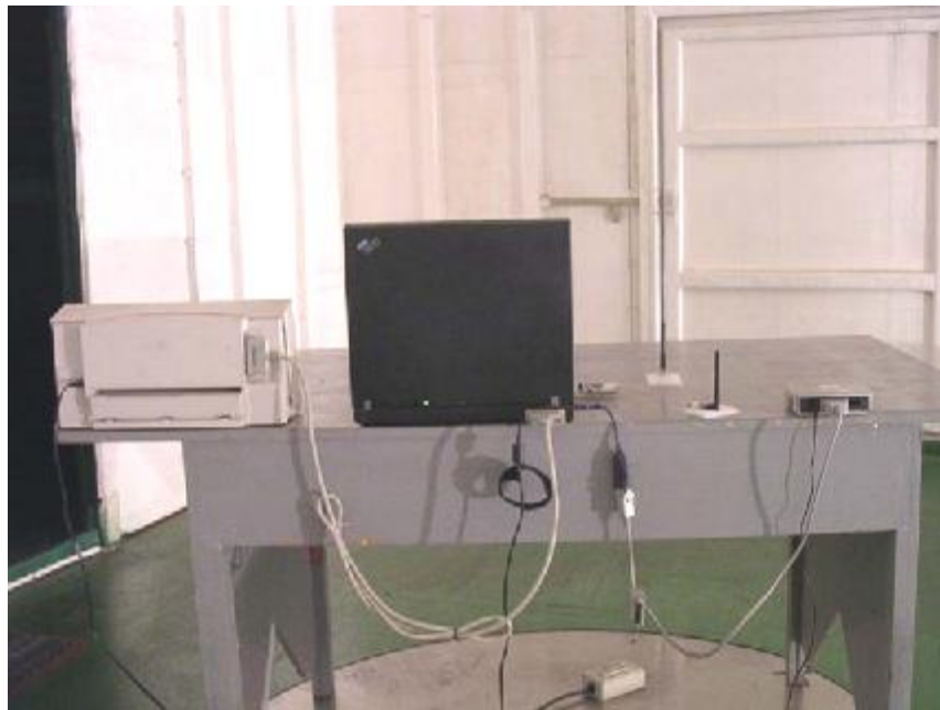
Photo 2: Radiated Emission Test Set-up
