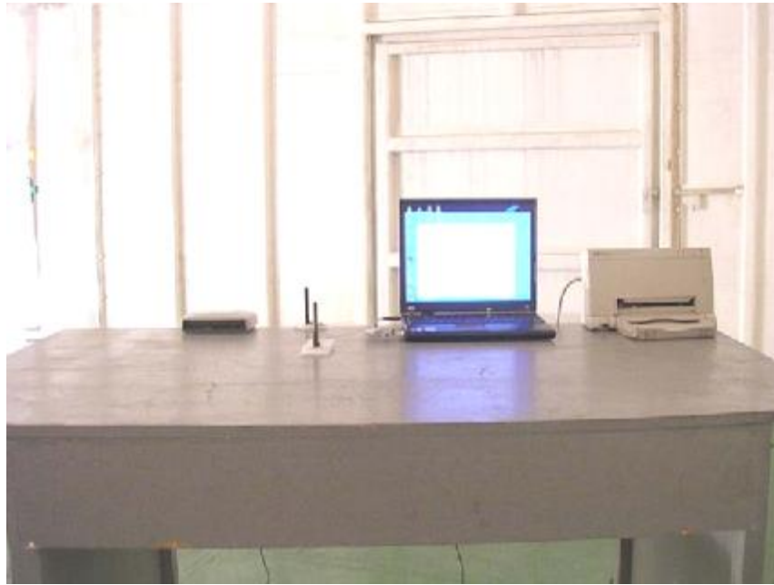
Photo 2: Radiated Emission Test Set-up
