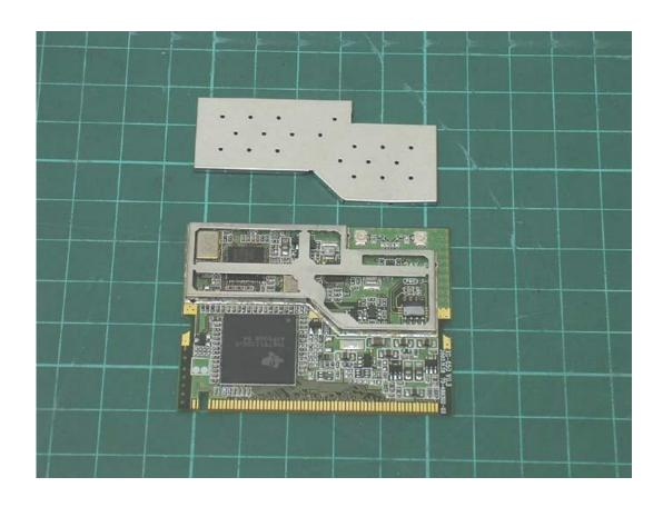
**Photo 2: Internal photo of EUT**
