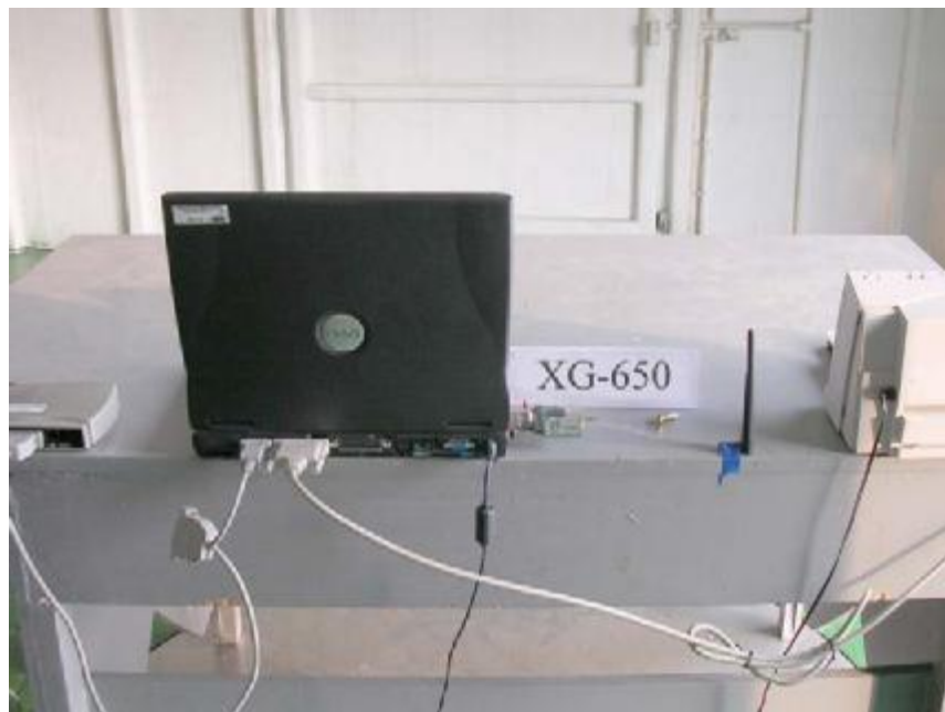
Photo 2: Radiated Emission Test Set-up
