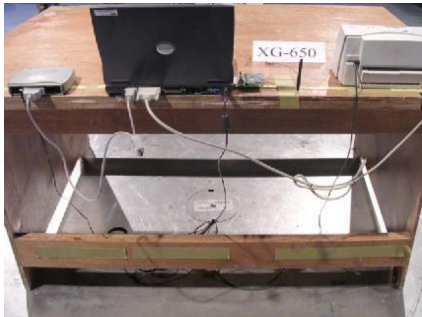
Photo 2: Radiated Emission Test Set-up
