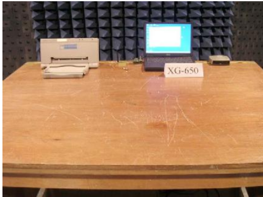
Photo 2: Radiated Emission Test Set-up
