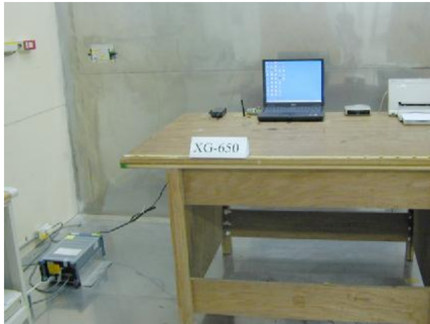
Photo 2: Conducted Emission Test Set-up
