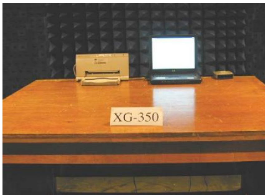
Photo 1: Radiated Spurious Test Set-up (front)
