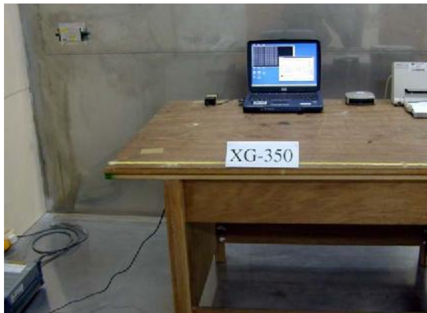
Photo 1: Conducted Emission Test Set-up (front)
