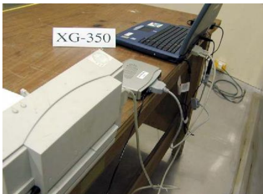
Photo 2: Conducted Emission Test Set-up (rear)
