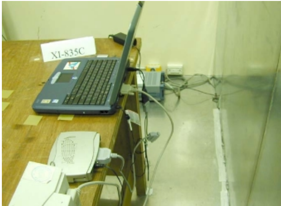
Photo 2: Conducted Test Set-up (rear)
