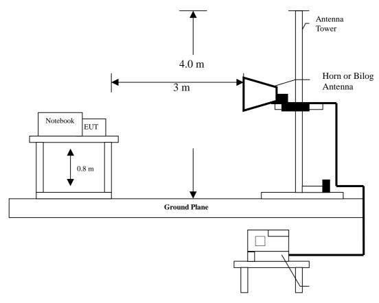
The signal is maximized through rotation and placement in the three orthogonal axes. The EUT and its peripherals are placed on a turn table which is 0.8 meter above ground. The turn table can rotate 360 degrees to determine the position of the maximum emission level. The EUT was positioned such that the distance from antenna to the EUT was 3 meters. The antenna can move up and down between 1 meter and 4 meters to find out the maximum emission level.
