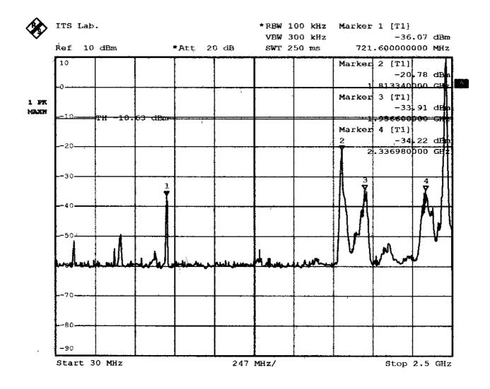
Comment A: RF conducted test at high channel Date: 2.JAN.2002 10:41:44
