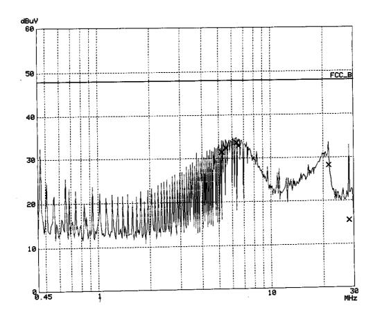
Intertek Testing Services RF VOLTAGE EUT: XI-325H Z-Com, Inc. AMN-L Manuf: Op Cond: Operator: Elton Test Spec: FCC 15 CLASS B SN:825788/015 120V 60HZ 22C 60%R.H TX mode at high channel Comment: 02. Jan 02 14:31 Date: Scan Settings (1 Range) StartStopStepIF BWDetectorM-TimeAttenPreamp450k30M8k9kPK20msAUTO LNOFF Final Measurement: x QP Meas Time: 1 s
