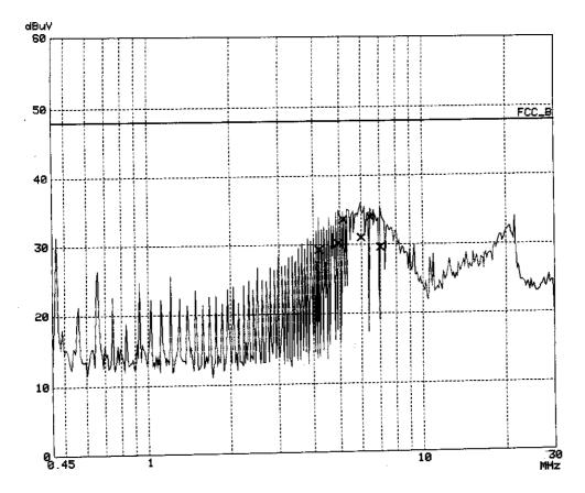
Intertek Testing Services RF VOLTAGE EUT: XI-325H Z-Com, Inc. Manuf: AMN-N Op Cond: Elton **Operator:** FCC 15 CLASS B SN:825788/015 120V 60HZ 22C 60%R.H TX mode at high channel 02. Jan 02 14:38 Test Spec: Comment: Date: Scan Settings (1 Range) Step IF BW Detector M-Time Atten Preamp 8k 9k PK 20ms AUTO LN OFF |------ Frequencies --Start Stop Stop 30M 450k Final Measurement: x QP Meas Time: 1 s
