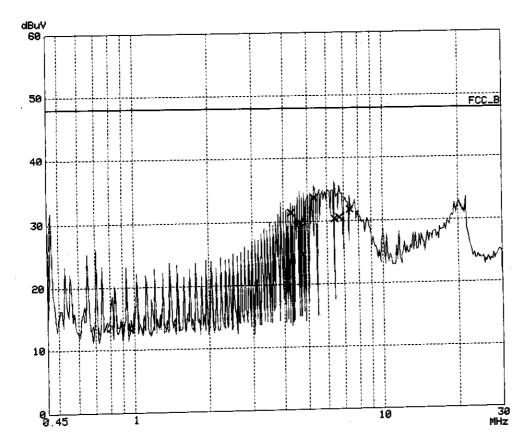
Intertek Testing Services RF VOLTAGE EUT: XI-325H Z-Com, Inc. Manuf: Op Cond: AMN-N **Operator:** Elton FCC 15 CLASS B SN:825788/015 120V 60HZ 22C 60%R.H TX mode at middle channel Test Spec: Comment: 02. Jan 02 14:18 Date: Scan Settings (1 Range) StartStopStepIF BWDetectorM-TimeAttenPreamp450k30M8k9kPK20msAUTO LNOFF Final Measurement: x QP Meas Time: 1 s
