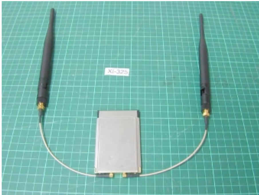
Photo 2: EUT with antenna (antenna gain is 5dBi)
