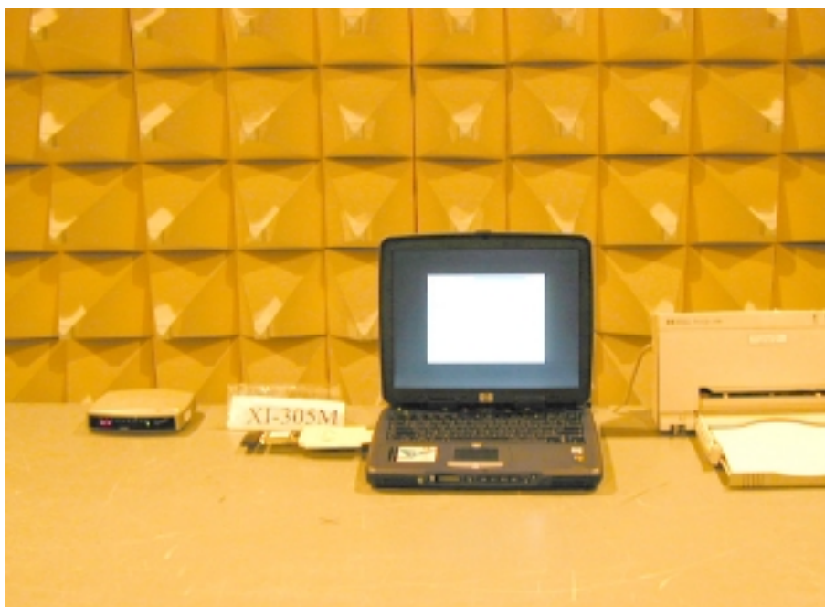
Photo 1: Radiated Emission Test Set-up (with Antenna 1)
