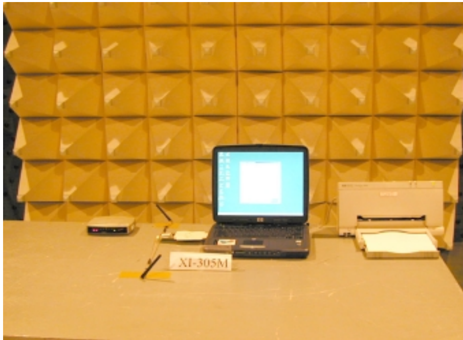
Photo 3: Radiated Emission Test Set-up (with Antenna 3)
