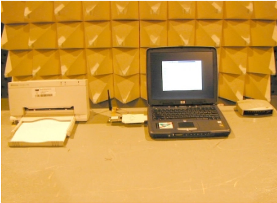
Photo 2: Radiated Emission Test Set-up (with Antenna 2)
