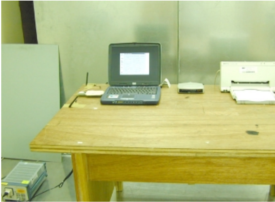
Photo 3: Conducted Emission Test Set-up (with Antenna 3)
