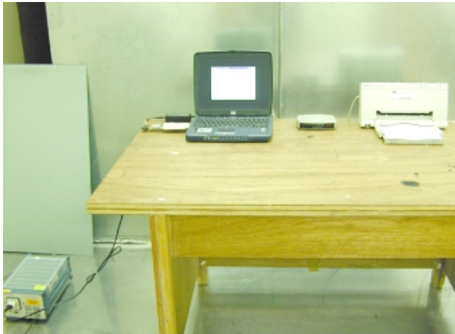
Photo 1: Conducted Emission Test Set-up (with Antenna 1)
