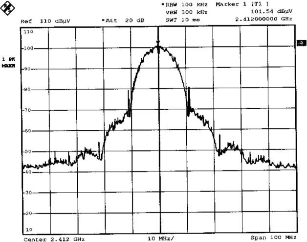
Comment A: RF conducted spurious at low channel with antenna A tx 11.JUN.2002 15:54:08 Date:
