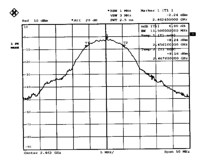
Comment A: 6 dB bandwidth at high channel with antenna A tx Date: 11.JUN.2002 15:10:12
