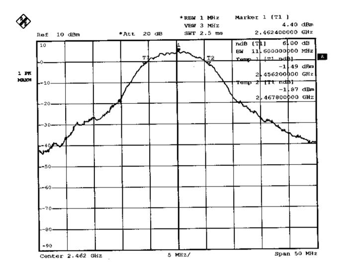
Comment A: 6 dB bandwidth at high channel with antenna B tx Date: 11.JJN.2002 12:58:07
