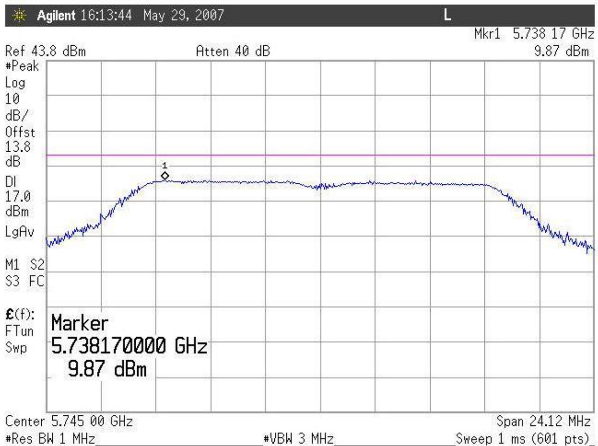
Figure 4-7. Peak Power Spectral Density, Low Channel
