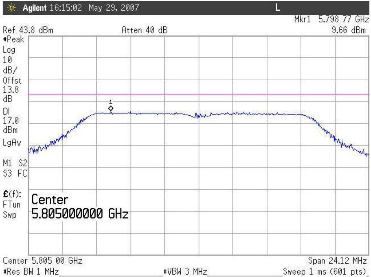
Figure 4-9. Peak Power Spectral Density, High Channel
