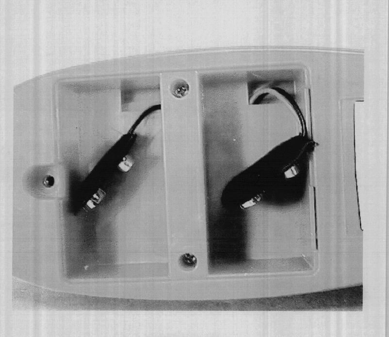
Battery Housing - two 9 VDC
