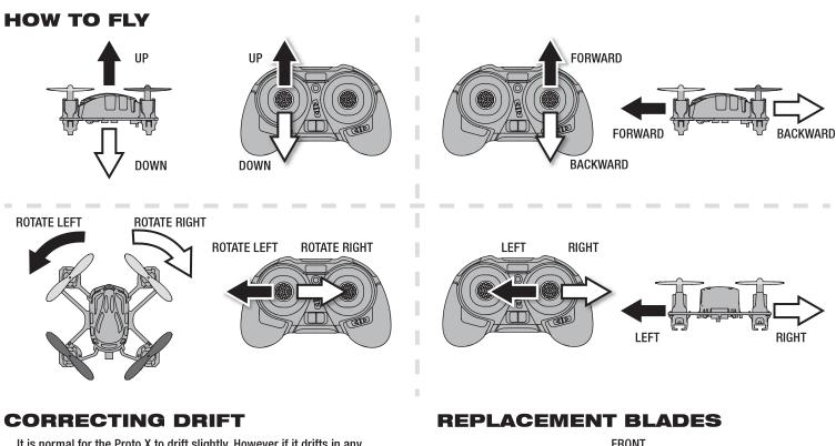
It is normal for the Proto X to drift slightly. However if it drifts in any direction consistently press the trim button opposite the movement as many times a needed to eliminate the drift.
