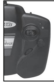
4. Charge until green LED turns off. Unplug cord and store in controller charge compartment.
