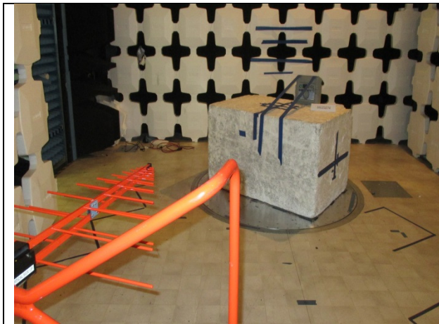
RADIATED FRONT PHOTO (BELOW 1 GHz)
