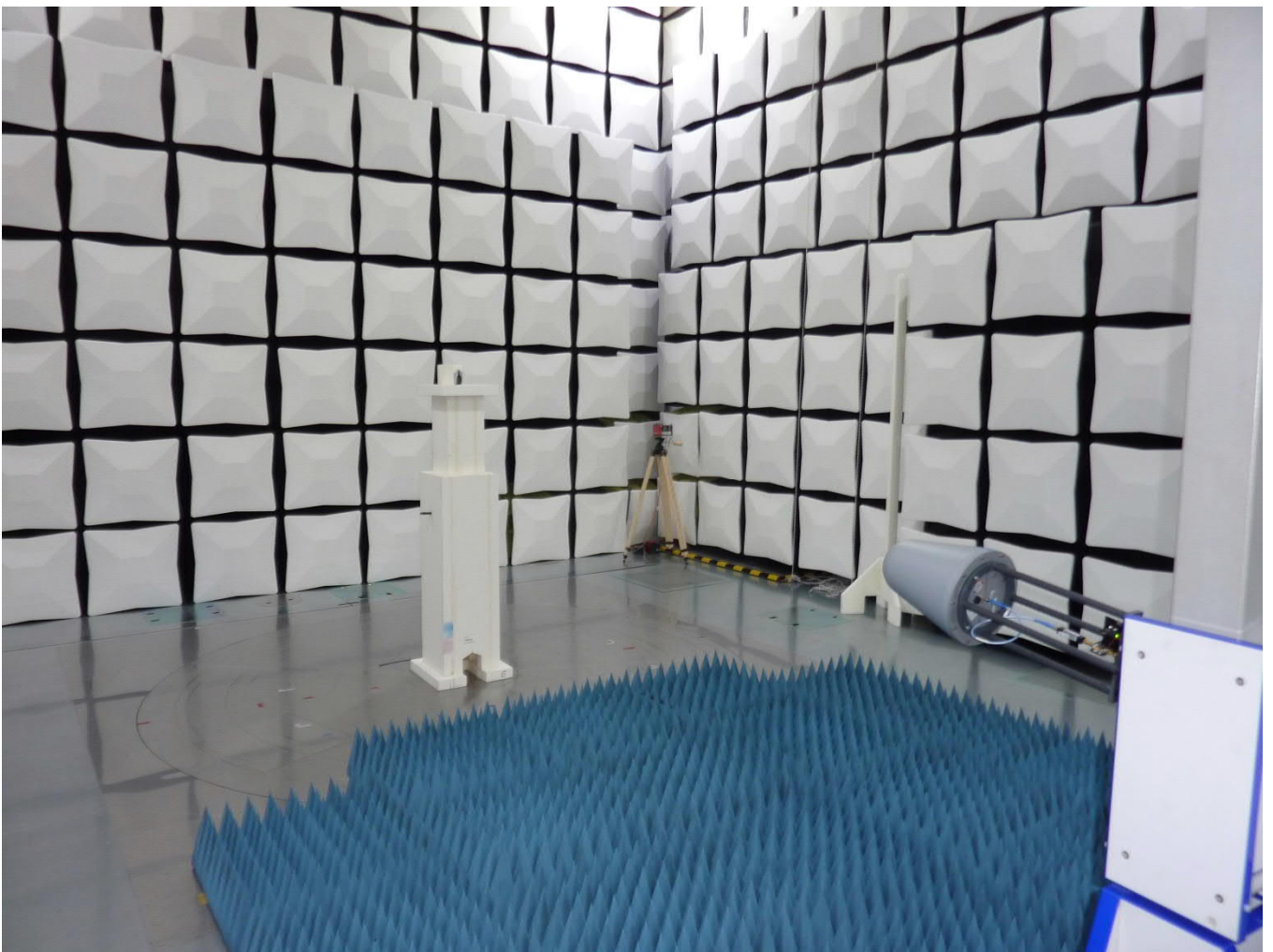
Test setup - Radiated emission 1 GHz to 4.5 GHz (semi anechoic chamber)
