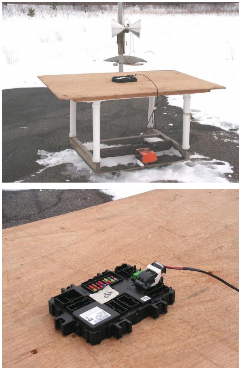
Figure 4: Radiated Emissions Test Setup Photograph(s).
