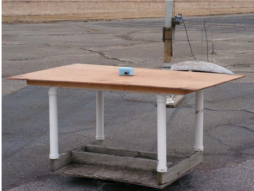
DUT on OATS – one of 3 axes tested
