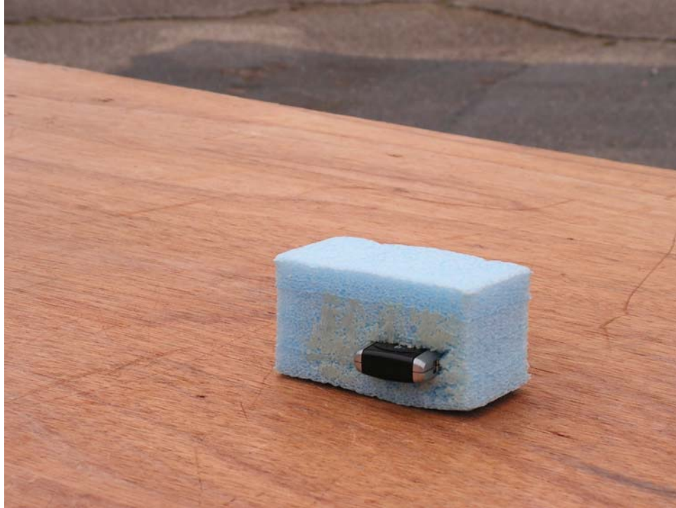
DUT on OATS (close-up) – one of 3 axes tested
