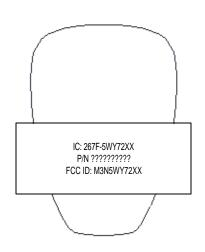
All information to be laser etched on rear side of housing. This will be performed at end of line test. P/N ?????????? refers to DaimlerChrysler part number to be assigned to this device.
