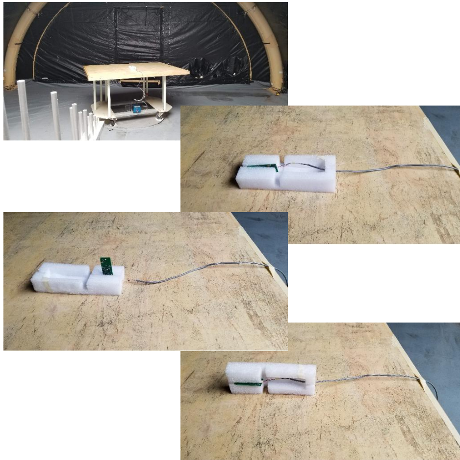
Figure 4: Radiated Emissions Test Setup Photograph(s).
