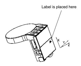
**Mechanical Drawing of the U152 IPATS Transceiver**
