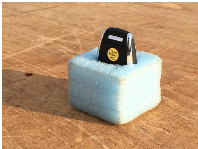
Figure 4: Radiated Emissions Test Setup Photograph(s).
