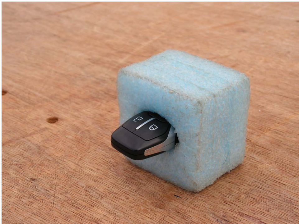
Photograph 6.6. Close-up of DUT on OATS (one of three axes tested)
