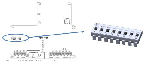
Figure 20 DIP SW S301, overview and detail
