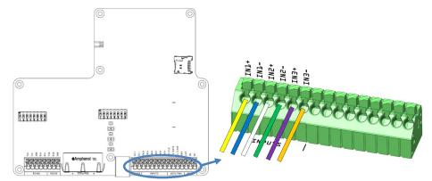
Figure 16 Input connections, overview and detail
