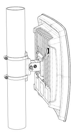
Figure 1 XT-1 mounted on a pole using UMK
