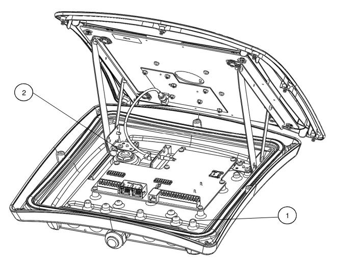
Figure 5 XT-1 overview (Pos. 1 is ground screw connection, Pos.2 is ventilating membrane)
