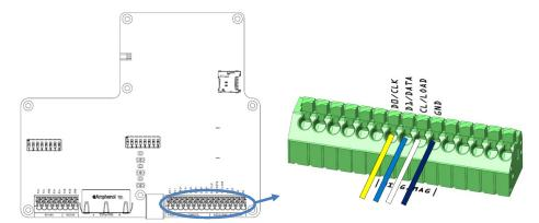
Figure 17 Output connections, overview and detail
