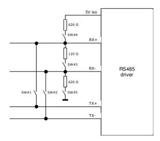
Figure 14 RS485 DIP switch configuration options
