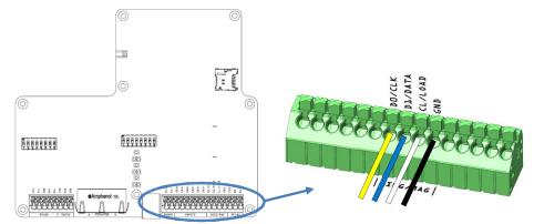
Figure 8 Wiegand connection, overview and detail
