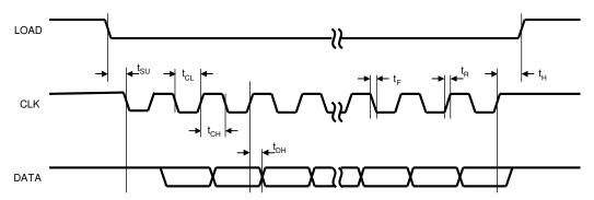
Figure 10 Magstripe timing diagram
