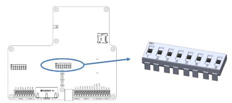
Figure 19 DIP SW S101, overview and detail
