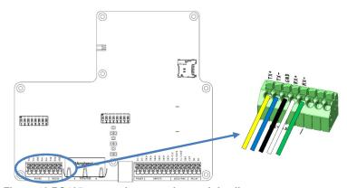
Figure 13 RS485 connection, overview and detail
