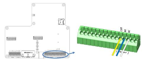
Figure 18 Relay connections, overview and detail
