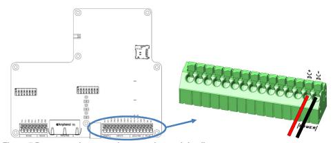
Figure 7 Power supply connection, overview and detail
