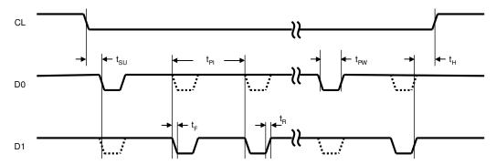
Figure 9 Wiegand timing diagram
