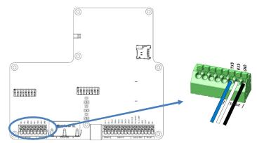
Figure 12 RS232 connection, overview and detail
