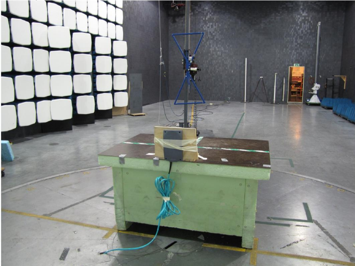
Test set up radiated emission 30 MHz – 1GHz
