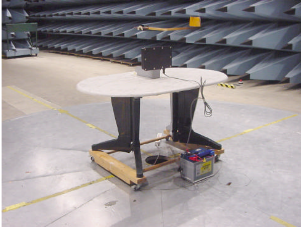
Semi-anechoic shielded chamber (30 - 1000 MHz), type S1566
