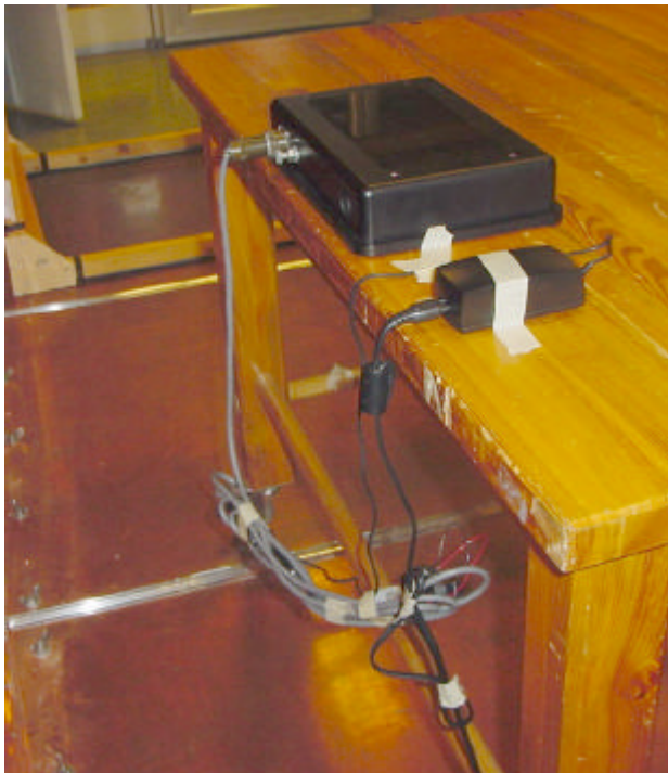
Conducted disturbance voltage 0,150-30 MHz, type S1566
