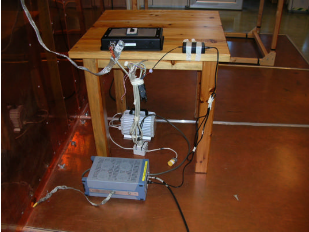
S1566 – Conducted disturbance voltage at AC terminal
