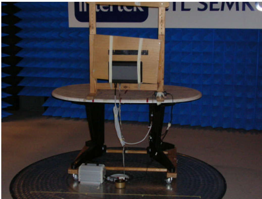
Model: S1566 - Radiated spurious emission 30-1000 MHz
