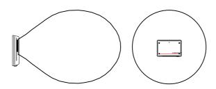
The reading and writing distances depend on the tag type and on the power and sensitivity SW settings. Typically, S1500 can read TagMaster tags at up to 6 m distance. See *Reading/Writing range* for details.
