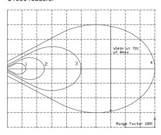
Curves 4, 3, 2 and 1 show areas for safe reading for the four different combinations of power and sensitivity.
