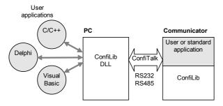
Communicator applications are developed in a PC environment with the cross compiler ConfiComp and can be executed in the PC for testing and debugging. The complete software is finally downloaded, using ConfiLoad, to the communicator for permanent storage in EEPROM. PC applications are developed with any PC software development tool. For application programmers a ConfiTalk Commander is available for training and low level communications management.
