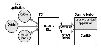
Reader applications are developed in a PC and the complete software is downloaded, using ConfiLoad, to the reader for permanent storage in EEPROM. PC applications are developed with any PC software development tool. For application programmers a ConfiTalk Commander is available for training and low level communications management.
