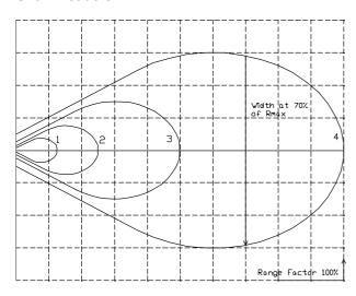
Curves 4, 3, 2 and 1 show areas for safe reading for the four different combinations of power and sensitivity.
