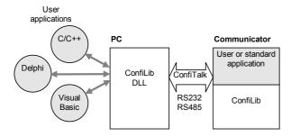
Reader applications are developed in a PC environment with the cross compiler ConfiComp and can be executed in the PC for testing and debugging. The complete software is finally downloaded, using ConfiLoad, to the reader for permanent storage in EEPROM. PC applications are developed with any PC software development tool. For application programmers a ConfiTalk Commander is available for training and low level communications management.
