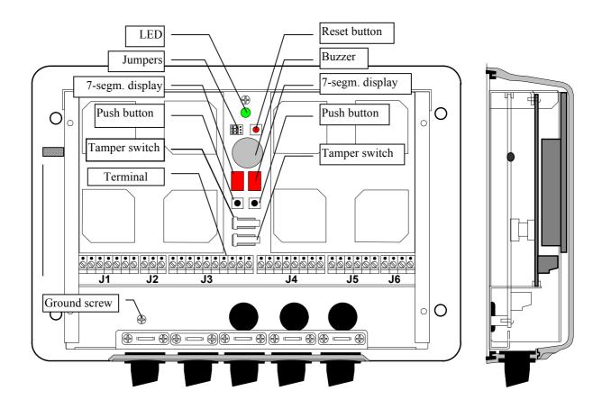
Connections to the Communicator are made using the terminal blocks J1 - J6.
