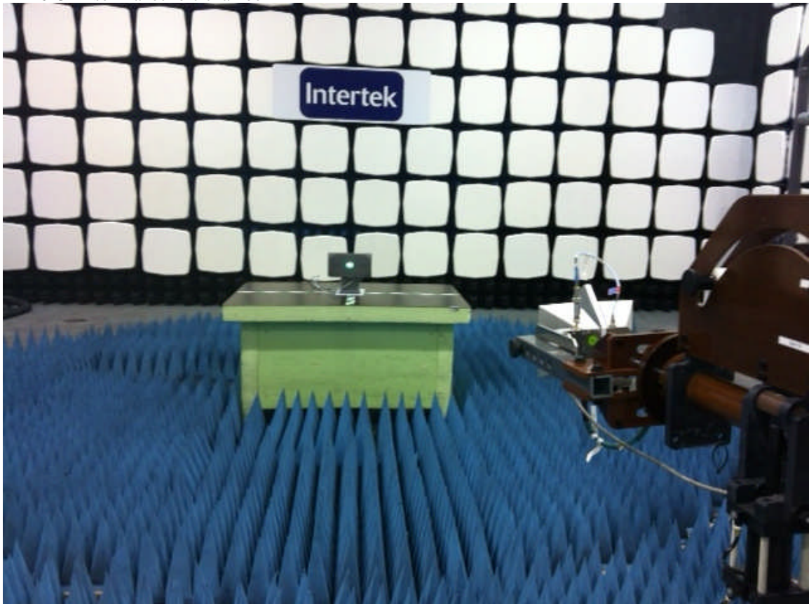
1 – 26 GHz semi anechoic chamber
