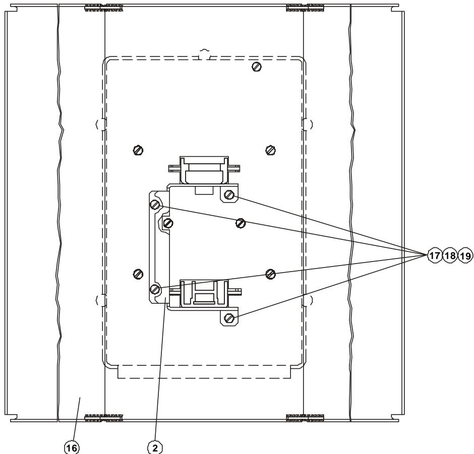
Figure 4-5. Tilt Holder Attachment
