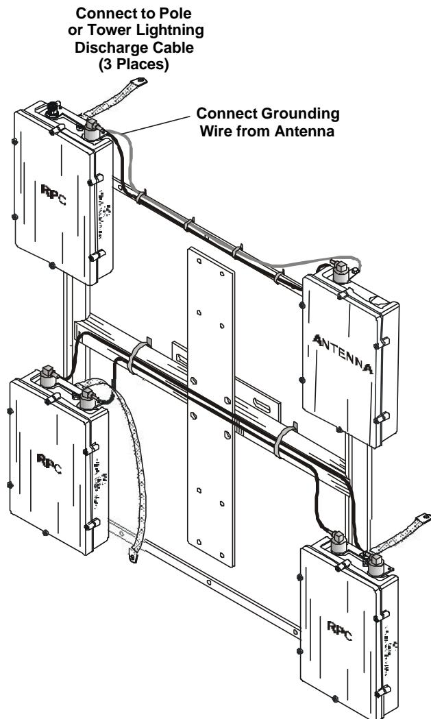
Figure 4-9. Two Dual-RPC and One Single-RPC Stations without Reflectors Mounted on H-Support
