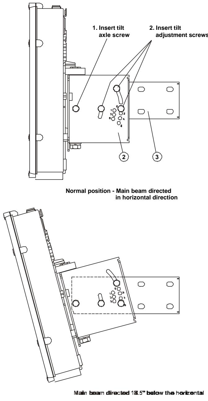
*Figure 4-6. RPC Tilt Adjustment*
