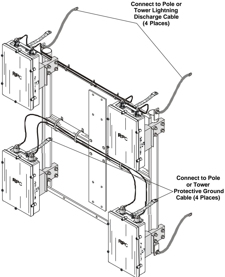
Figure 4-7. Four RPC's Mounted on H-Support
