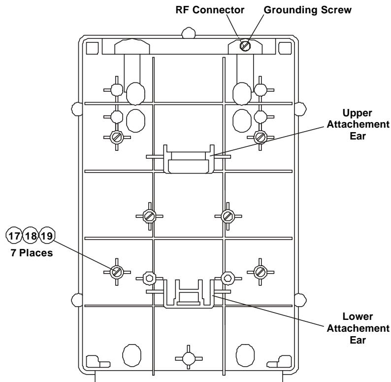
Figure 4-4. Attachment of Reflector
