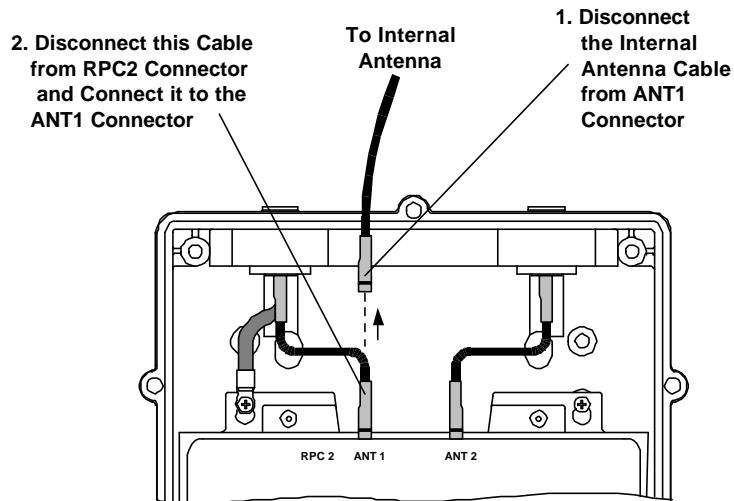
Figure 4-12. RPC Internal Connections for Operation with Two External Antennas
