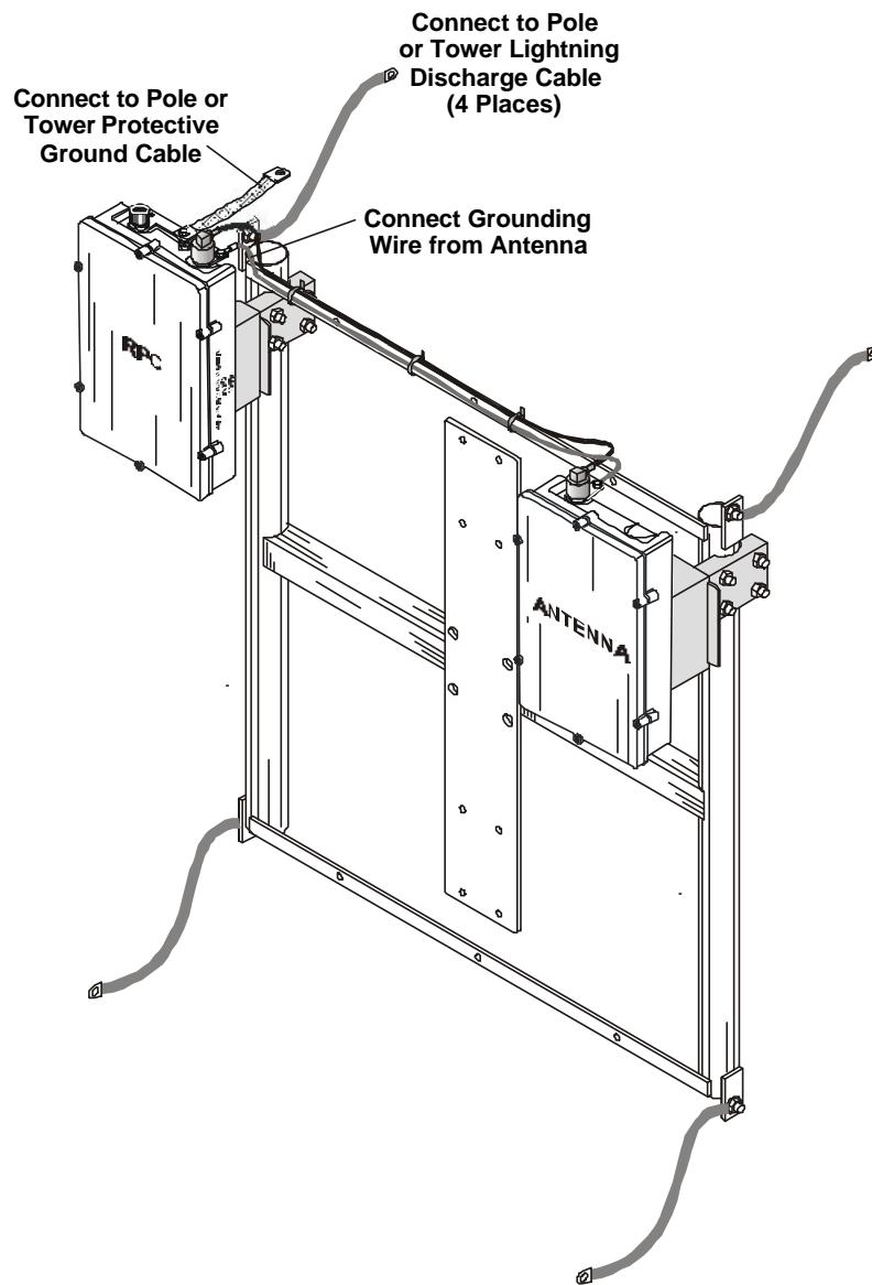
Figure 4-10. Single-RPC Station with One External Antenna Reflector Mounted on H-Support
