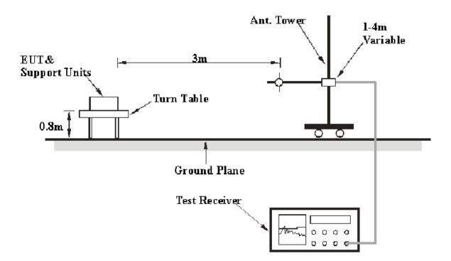
The radiated emission tests were performed in the 3 meters test site, using the setup accordance with the ANSI C63.17 - 2006. The specification used was the FCC 15.209 and FCC 15.319(g) limits.
