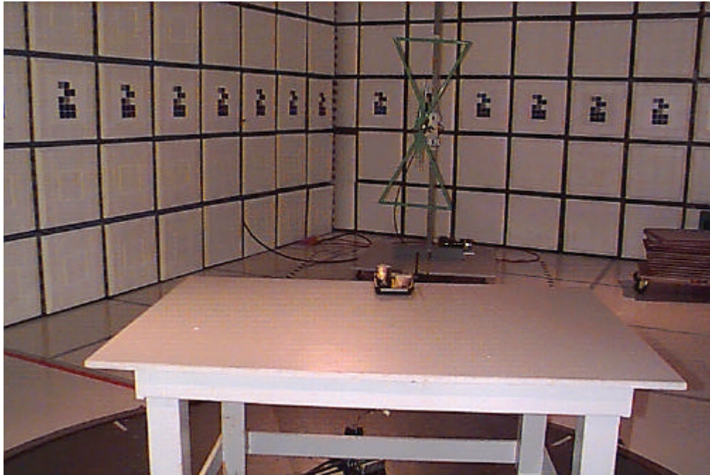
Radiated Emissions Test Set-up Front View
