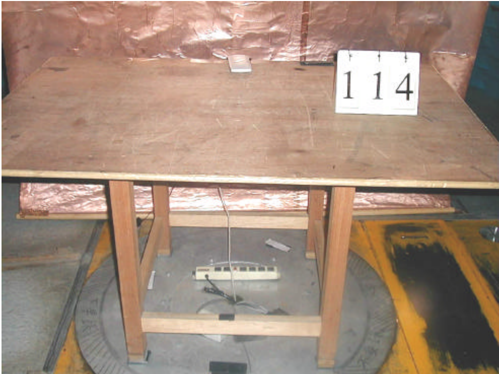
Conducted Emissions Test Placement
