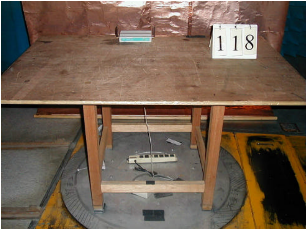
Conducted Emissions Test Placement (Power by AC Source)
