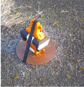
(c) Configuration 8 “Beacon above ground plane” as defined in Cospas-Sarsat C/S T.007 specification, ELiTe ELT is transmitting while kept away from ground (insulated, no need of ground plane).
