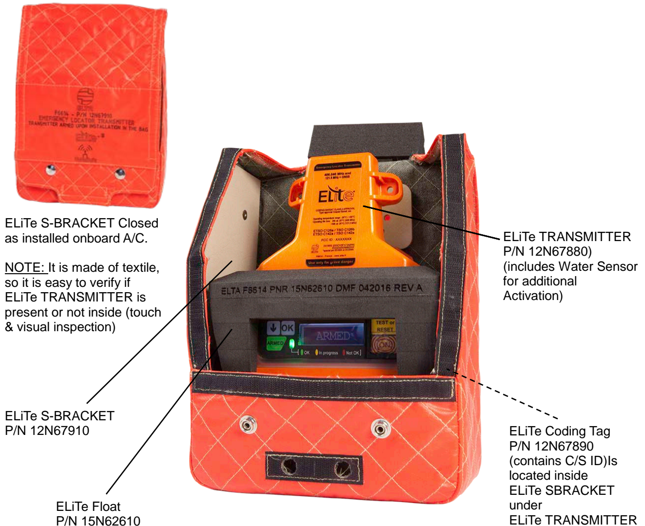
Figure 4 Survival – ELiTe S-BRACKET Sub Components
