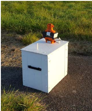
(c) Configuration 8 “Beacon above ground plane” as defined in Cospas-Sarsat C/S T.007 specification, ELiTe ELT is transmitting while kept away from ground (insulated, no need of ground plane).
