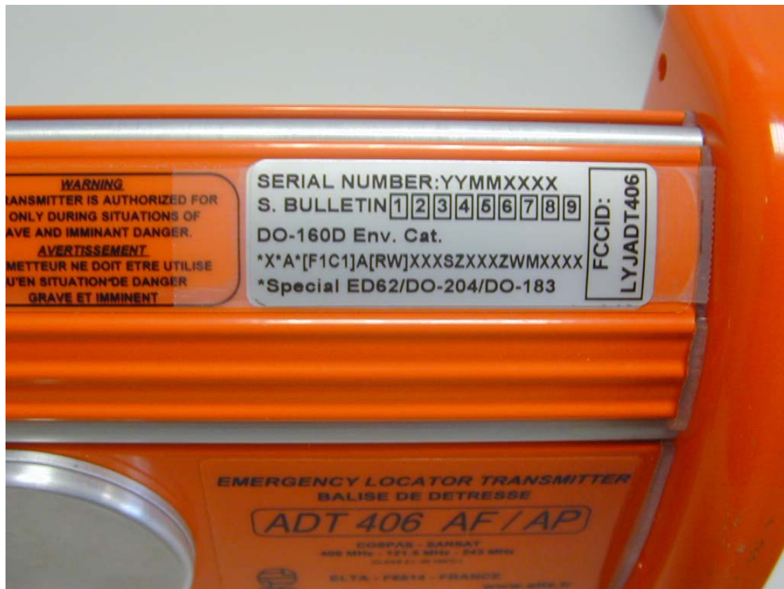
FCCID label content on ELT model ADT 406 AF-AP
