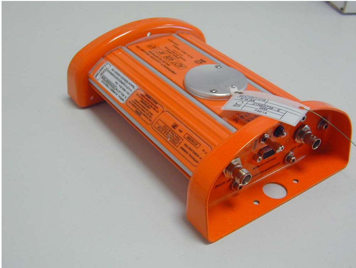
FCCID label location on ELT model ADT 406 AF-AP
