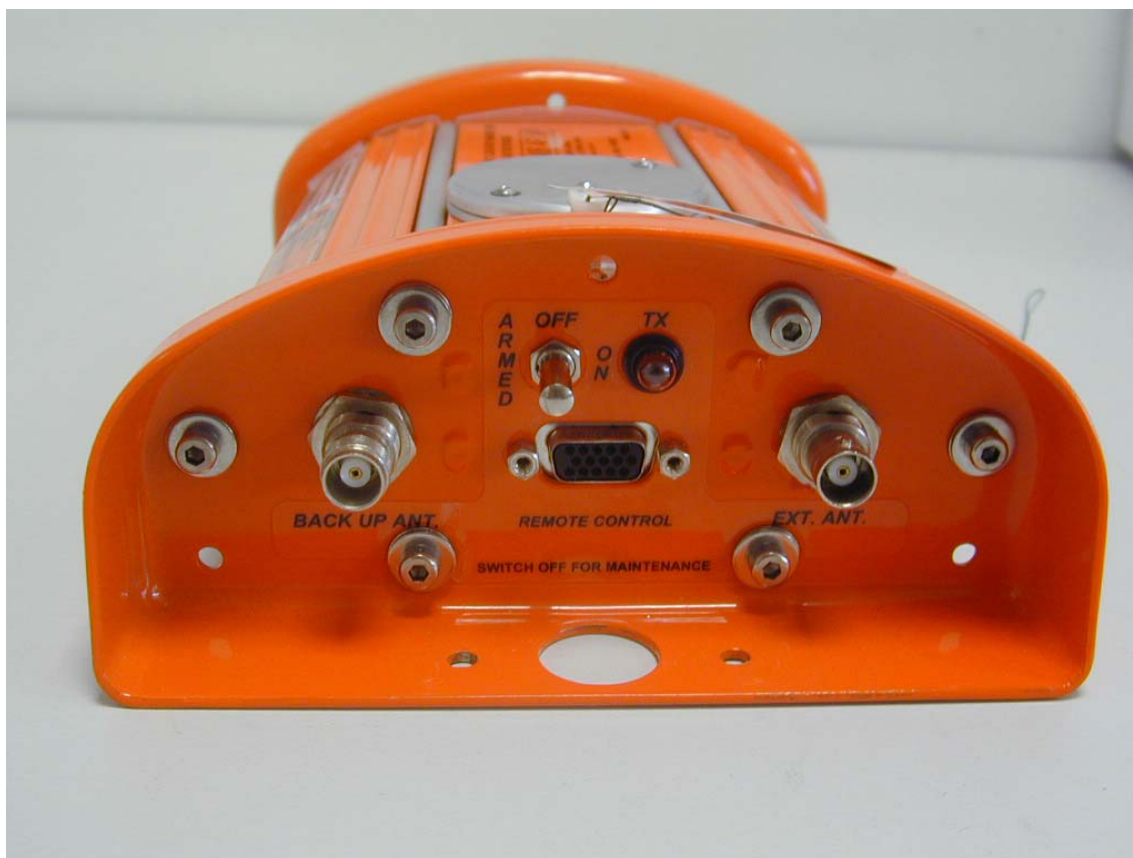
Control panel on ELT model ADT 406 AF-AP
