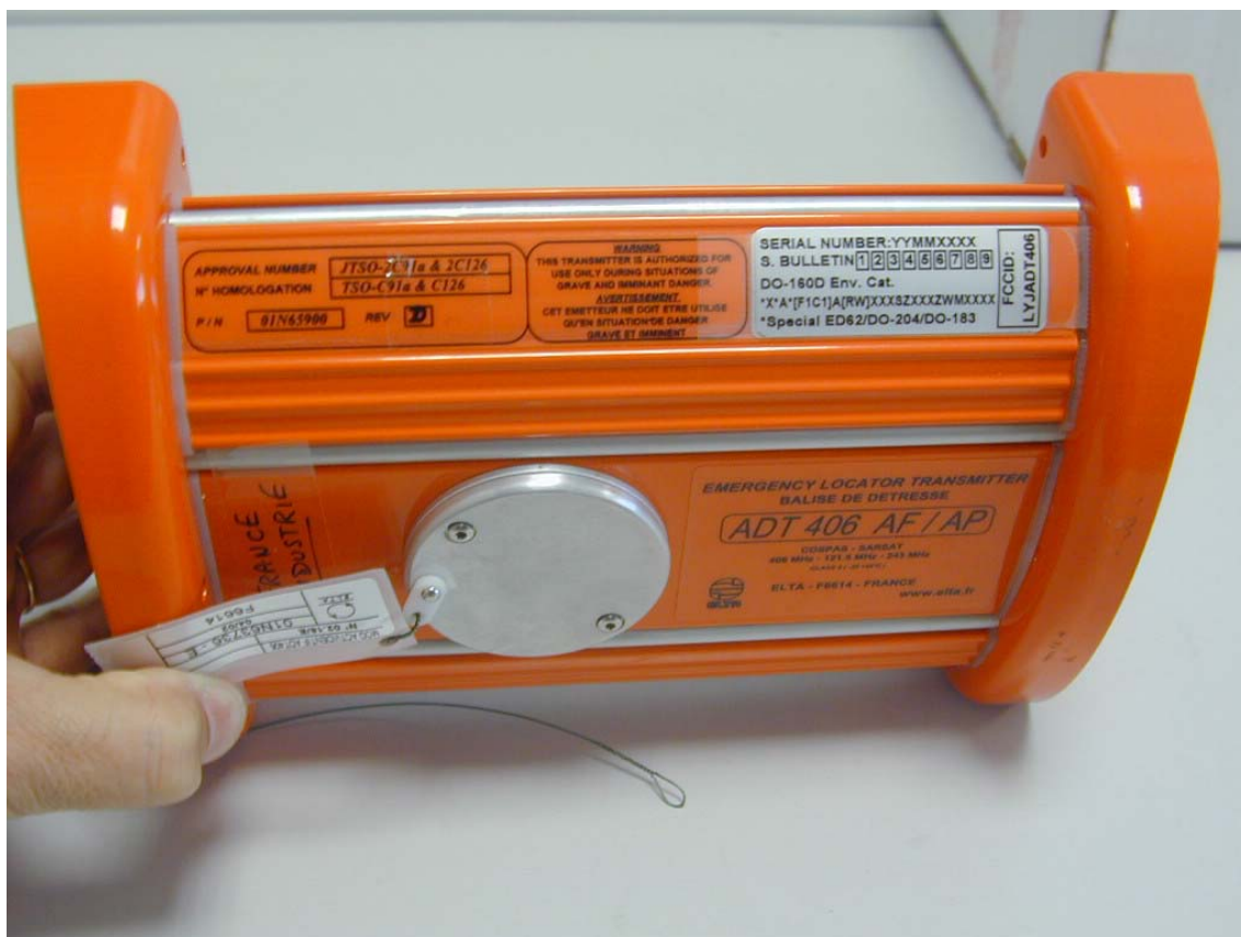
ID & FAA label location on ELT model ADT 406 AF-AP
