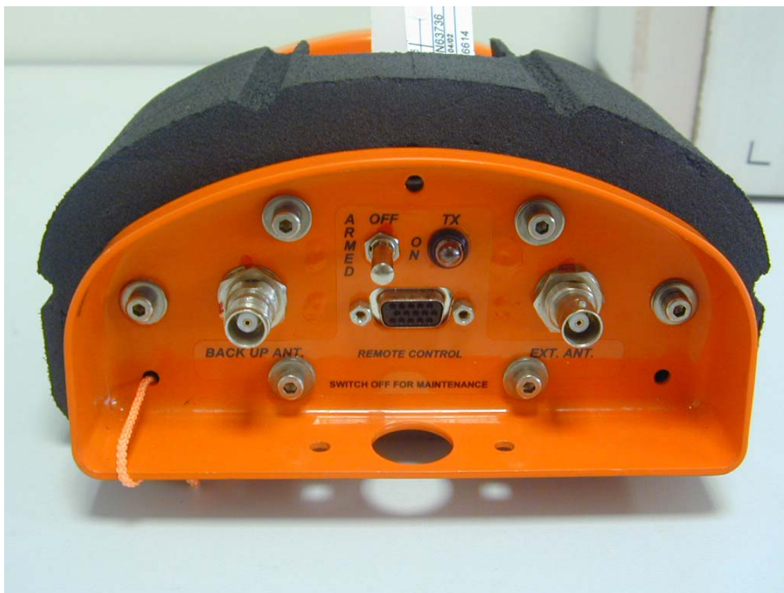
Control panel on ELT model ADT 406 AP
