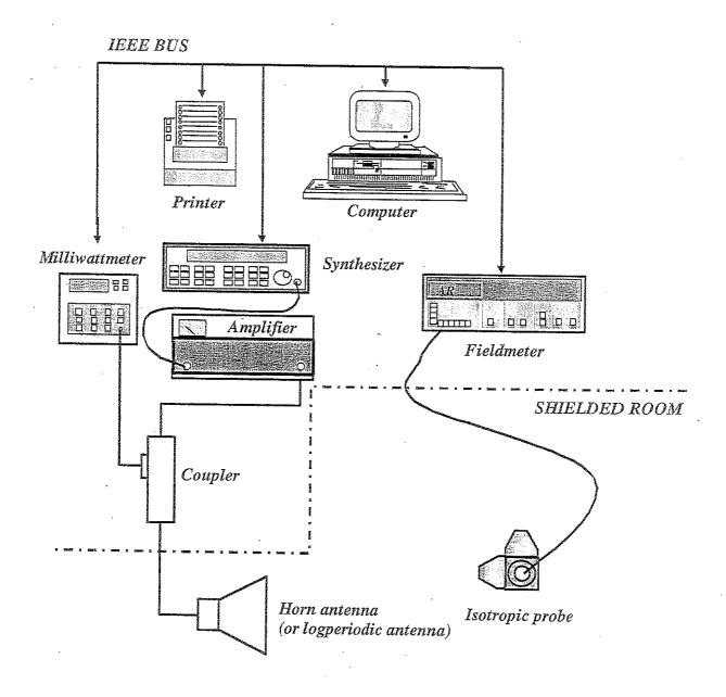
NB: From 1 GHz to 18 GHz, the coupler, the milliwattmeter, the amplifier and the synthesizer are placed inside shielded room.
