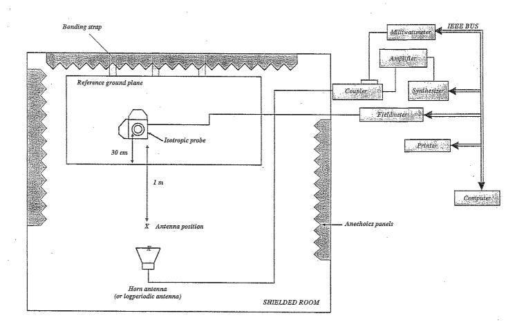
NB: From 1 GHz to 18 GHz, the coupler, the milliwattmeter, the amplifier and the synthesizer are placed inside shielded room.
