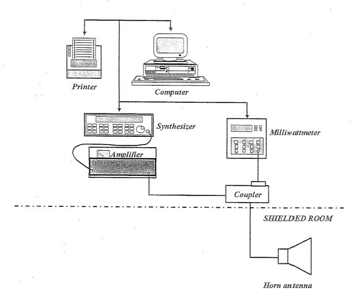
NB: From 1 GHz to 18 GHz, the coupler, the milliwattmeter, the amplifier and the synthesizer are placed inside shielded room
