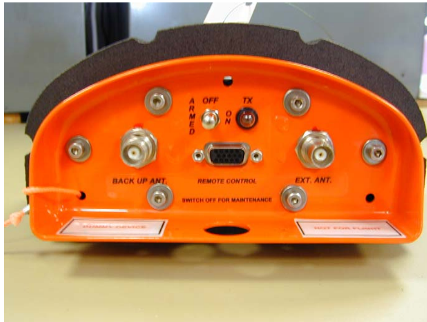
ADT 406 AP General view with its bracket mount, protective cover and secondary whip antenna
