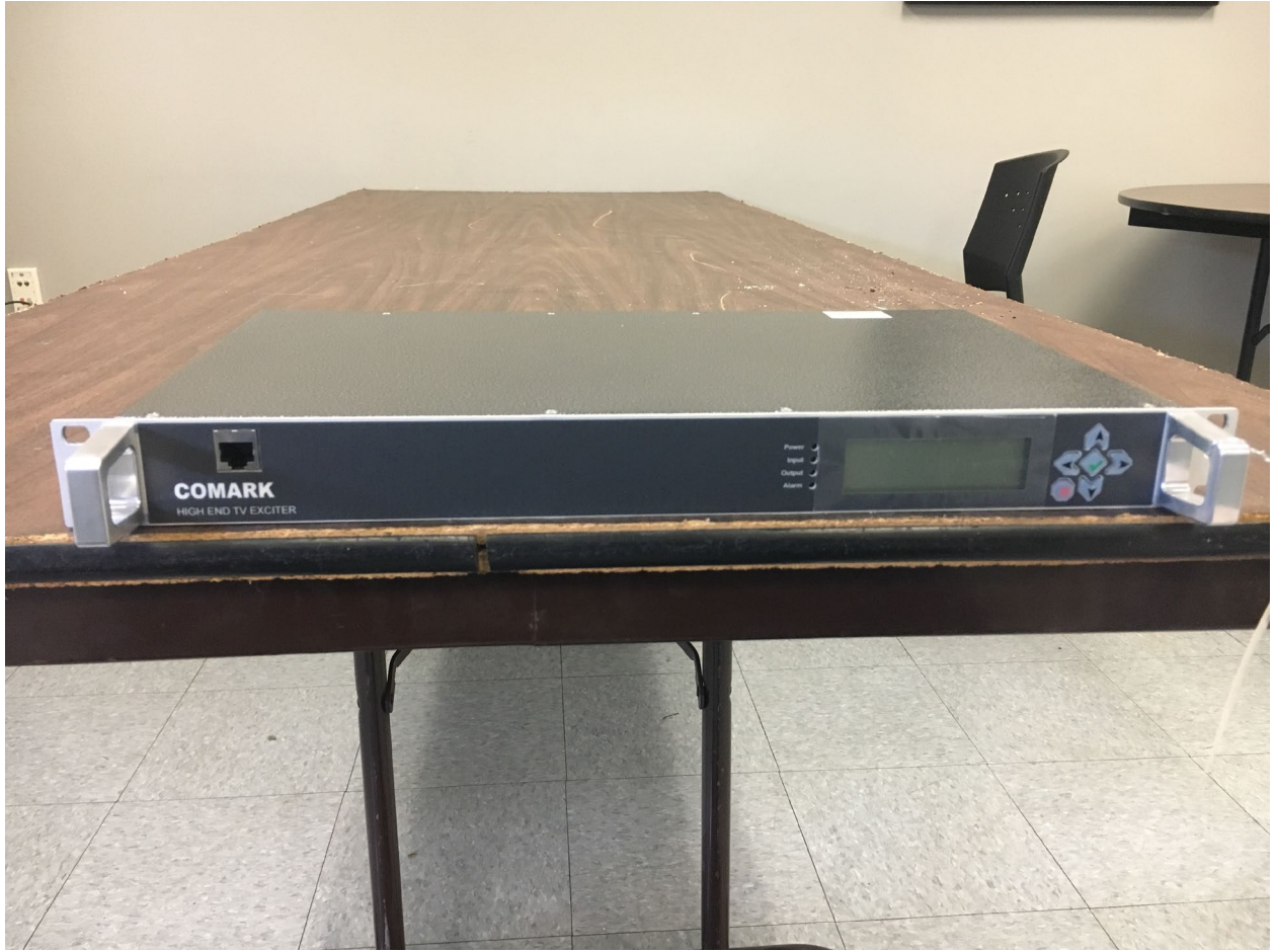
Figure 3. Exact V2 Exciter Front View
