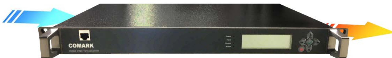
Figure 41: Rack air flow
