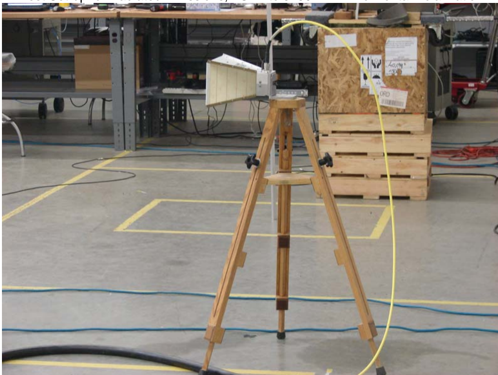
Test Set-up for Radiated Emissions, 1GHz to 5150MHz – Vertical Polarization
