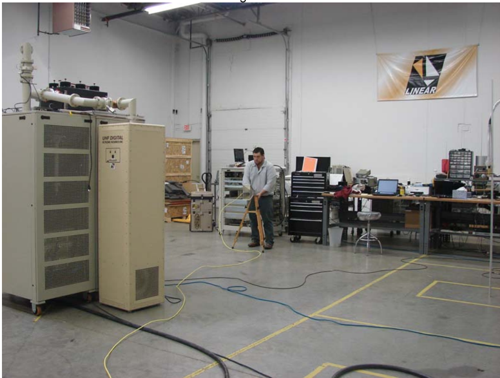
Test Set-up for Radiated Emissions, 1GHz to 5150MHz – Horizontal Polarization
